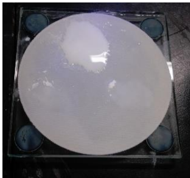
Figure 13. Grab a working Electrode and polish it while drawing "∞" on a polishing pad.
